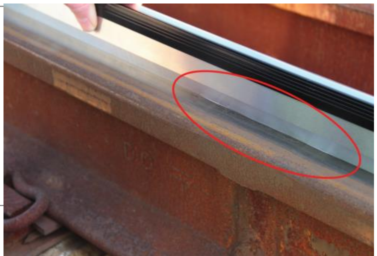
Fig. 4: Dents caused by wear in the annealing zone of a thermite weld
