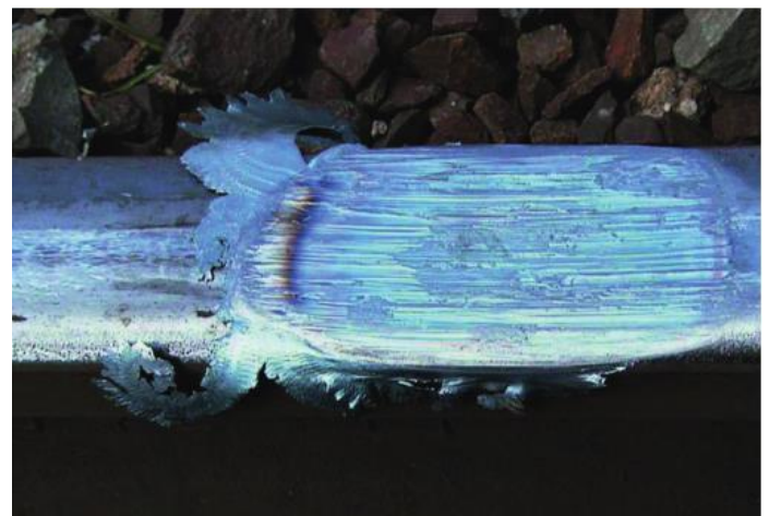
Fig. 1a/1b: Repair, don't throw away: Head checks ("oblique") and deep wheel slip marks, which normally require a closure rail replacement, can be repaired or built up and optimised with automated GMAW welding
