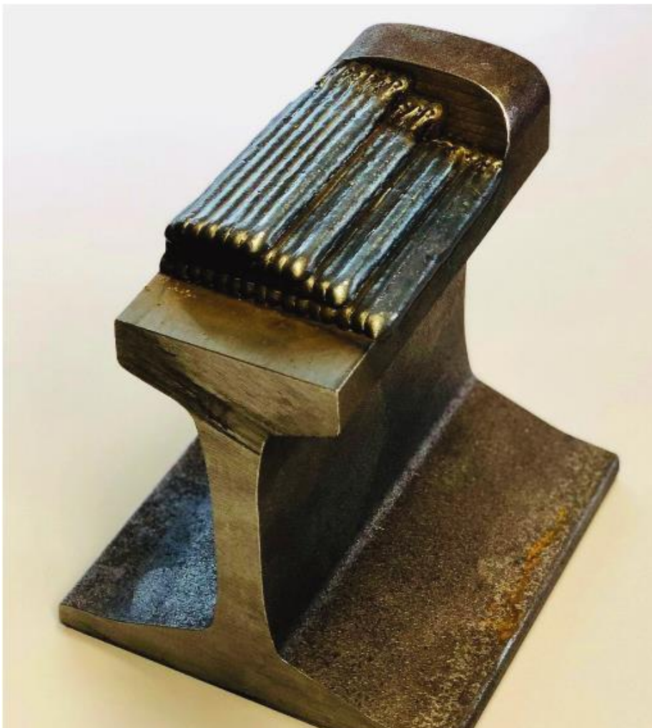
Fig. 6: Instead of replacing parts, the original geometry is reconstructed quickly in layers and thus completely reinstated.
